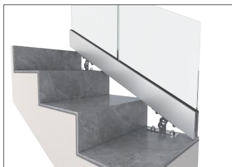
楼梯安装 Detail of Stairway Application
